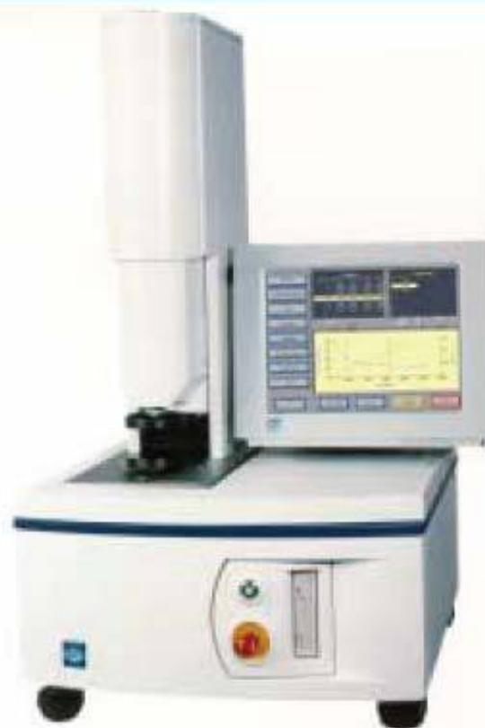
The Lab Master® Softness Tester provides precise measurement of bulking thickness and compressibility. Manufacturers and specifiers of tissue, nonwoven and textile products are now able to measure softness to an objective standard. Softness Index correlates to test panel evaluations of softness.
