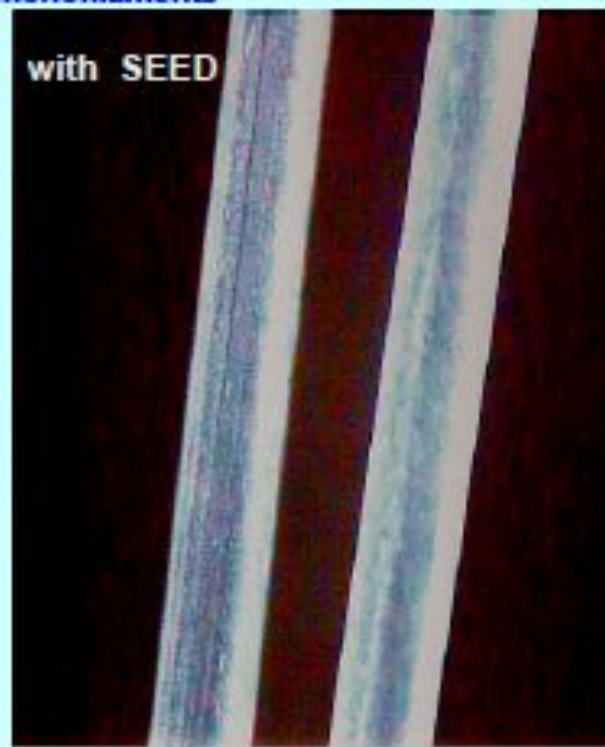
Microphotography of PA monofilaments
