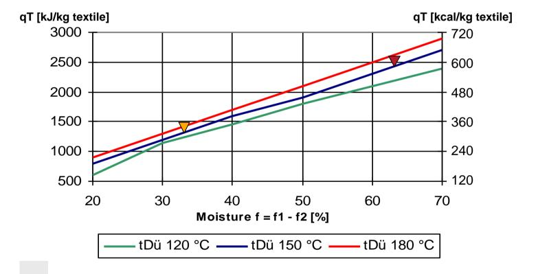
Example 1 pick-up = 70%, residual moisture = 8% q<sub>T</sub> 2400 kJ/kg textile
